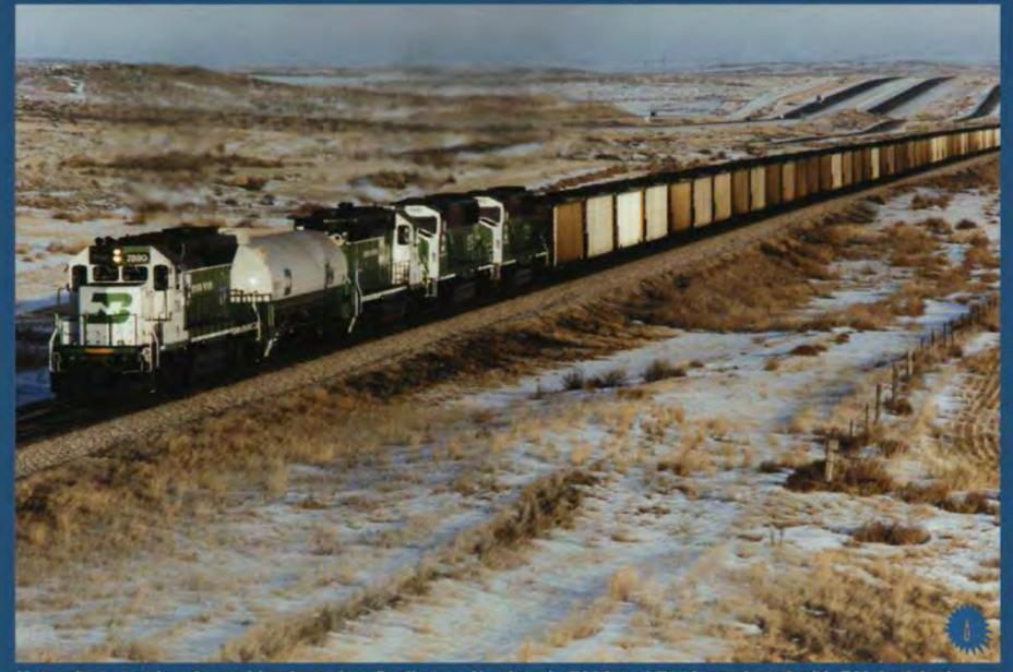
Natural gas tandem in coal haul service. Burlington Northern's 7890 and 7149, equipped with ECI dual-fuel conversion systems. The locomotive pair, coupled to the 20,000 gallon LNG tender car, achieves full power and has a range of more than 800 miles between refueling.
